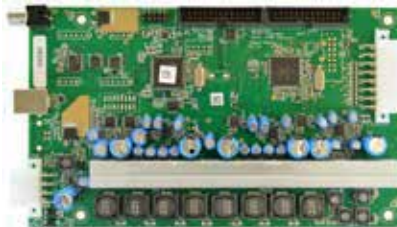
The multi-channel Class D amplifier features advanced Digital Signal Processing (DSP) for superior sound quality
