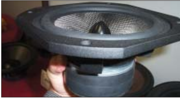
PHOTO 6: MISCO is traditionally known for its small full-range speakers, but also produces high-end woofers with advanced materials and features, such as this 8" bass midrange.
