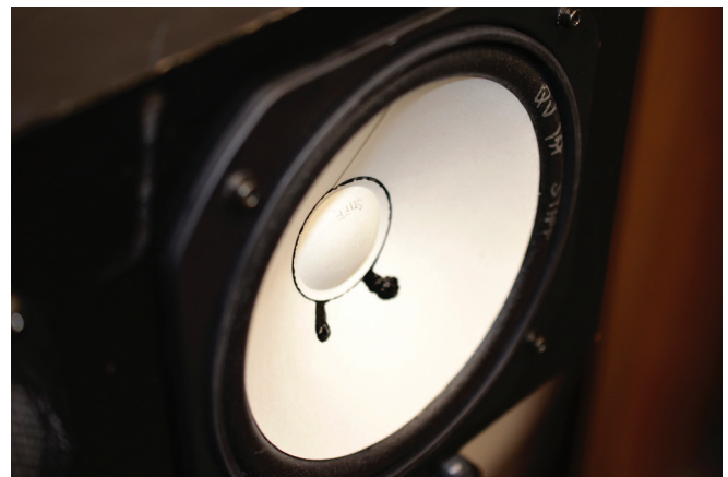
MS10-W prototype mounted in NS10M enclosure. Note the cone seam.
