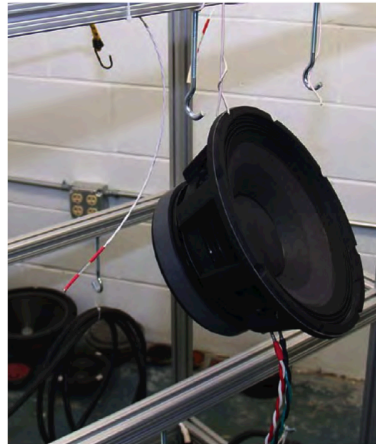
Power testing a high-performance woofer in free air.
